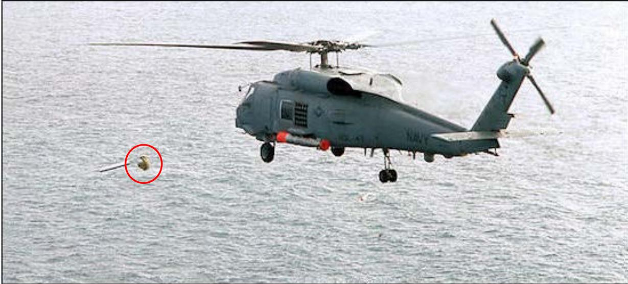
**Figure 3.0-1: Sonobuoy Launch Depicting the Relative Size of a Small Decelerator/Parachute**
