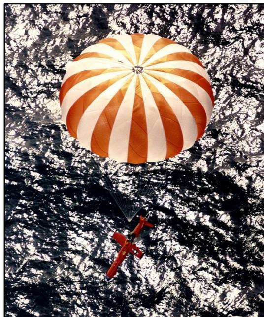
**Figure 3.0-2: Aerial Target (Drone) with Parachute Deployed**
